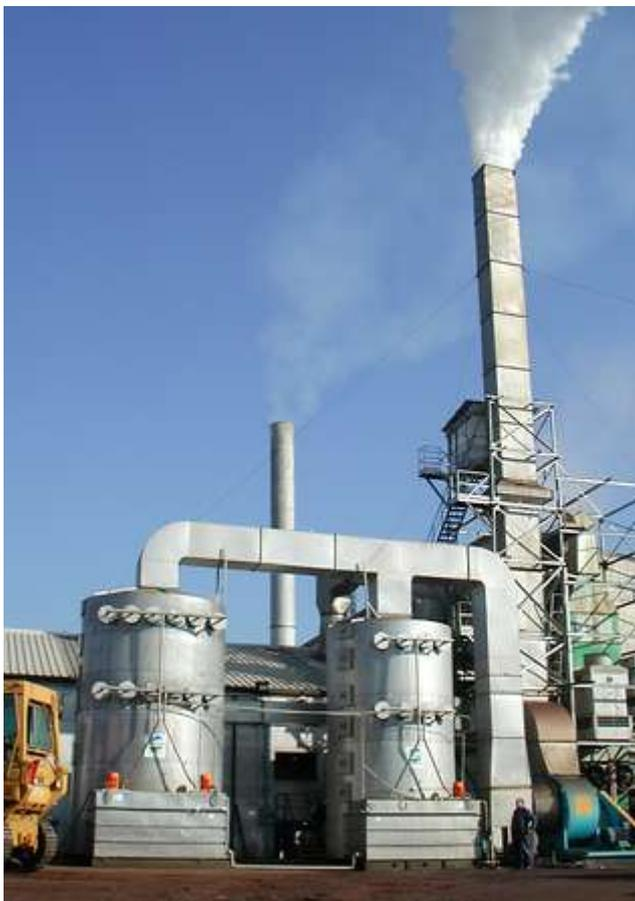
This system is made up of two vertical wet scrubbers, as the capacity of the air to be treated is very high. The system has been made up of stainless steel, in order to ensure higher resistance
