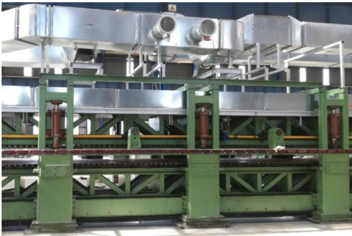
The machine structure was completed with the application of the upper/lower covers in galvanized metal sheets used to avoid heat loss.
