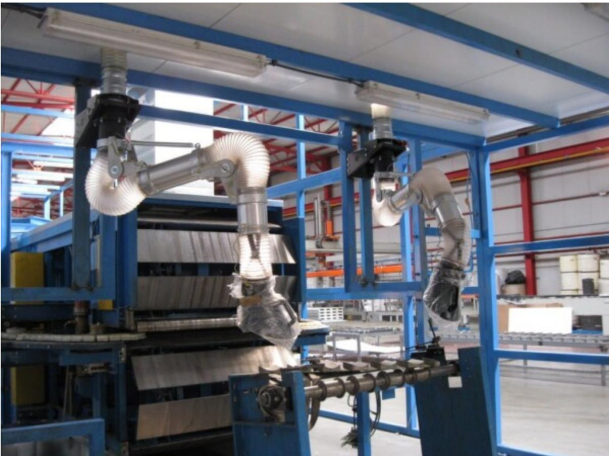
As we have seen, **pentane** is used in the **foaming step** of production: it is an expanding agent characterized by a strong odor (similar to gasoline) and a certain volatility (it keeps its liquid phase up to 36,1 °C, then start boiling). Pentane vapors are extremely flammable and can create a potentially explosive atmosphere.
