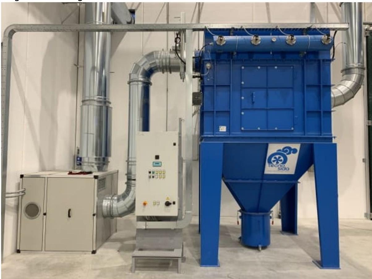
The bag or cartridges filters are systems that, instead of exploiting laws of physics such as centrifugal force, utilize a filter media to purify the air and retain polluting particles.
