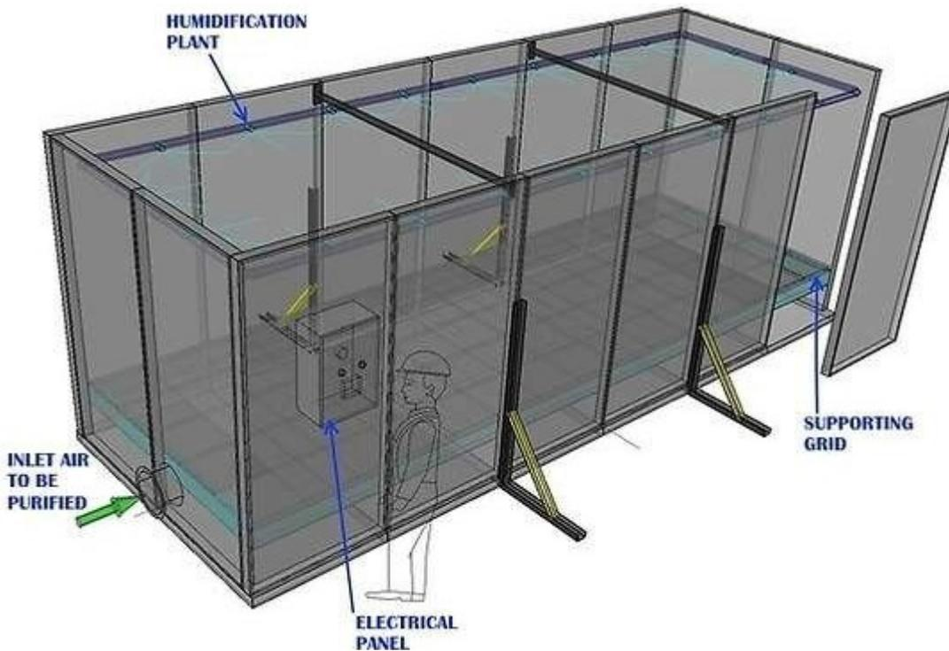
In order to obtain a good functionality of the biofilter, is essential to create an habitat that is adequate for the development of the microflora. In particular:
